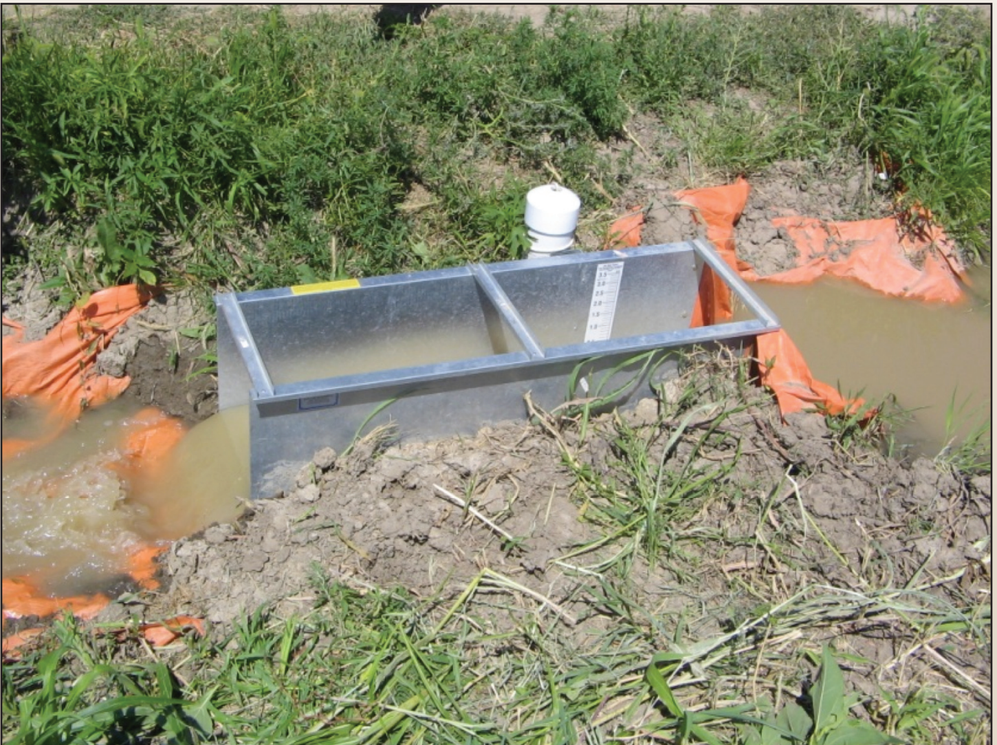
Figure 12. EZ Flow Ramp™ flume used to measure tailwater from field DS14 during 2005 and 2007
